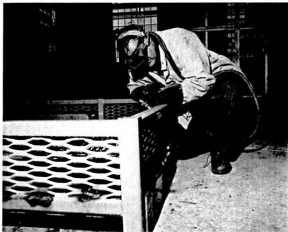
This JUT41 scissorlift is being prepared by maintenance crews at Levack mine for transfer to a 3400-foot level cut-and-fill stope where it will be used for installation of roof bolts, wire mesh, ventilation pipe, compressed air and water lines and for the loading of explosives. Fitted with an elevating platform, eight feet wide and 12 feet long, the deck has a 2,000 pound carrying capacity when in the elevated position, which reaches as high as eight and a half feet from the ground. Above, maintenance mechanics Robert Dionne , Don Shannon and Bert Houle prepare the unit for its move underground. Below, plater Clifford Cardinal puts the finishing touches on the platform.
