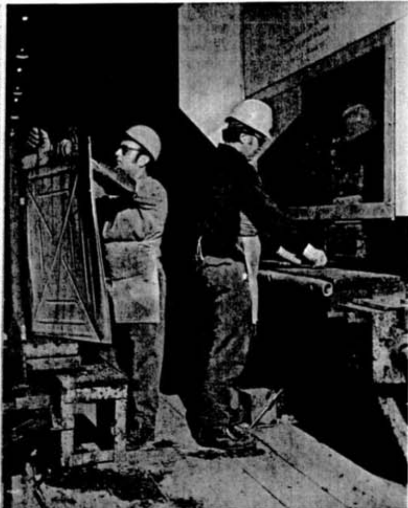
Biagio Crognale feeds a nickel cathode sheet through as Tony DiNunzio "walks" another sheet from the rack. The cut strips then travel by conveyor belt to No. 6 shear where they are cut into squares and packed into drums.
