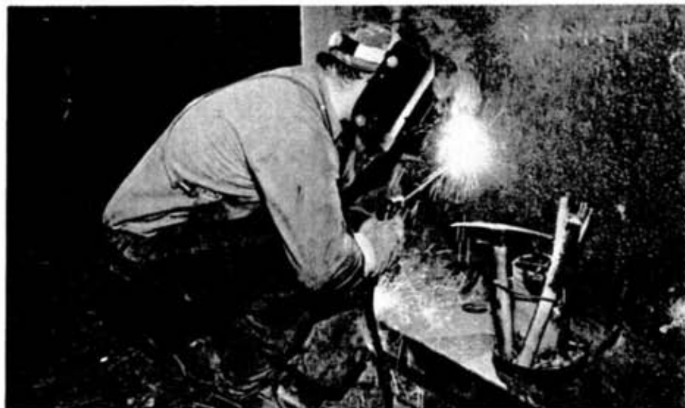
Yves Lariviere, specialist welder, carefully welds a small crack on the upper frame section of the Kirkwood crusher, which will be used as a replacement unit at Garson mine.
