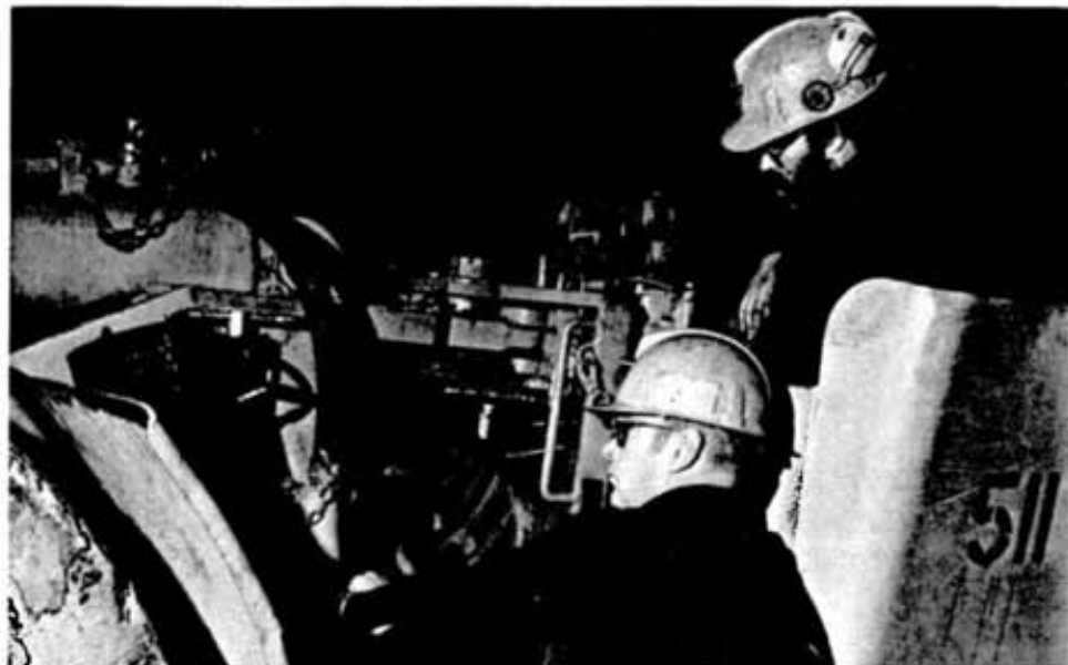
Following installation and testing, Chuck Briggs, foreground, and scooptram operator, Terry Short, adjust the fire suppression system's main supply tank.
