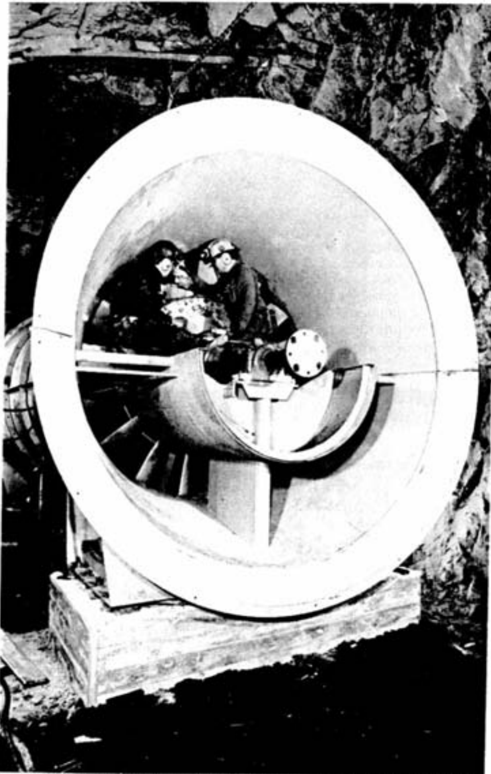
Brent Holmes, left, and Karl Neuman, Creighton mine ventilation assistants, adjust the fan blade settings, one of the methods of controlling fan performance.
