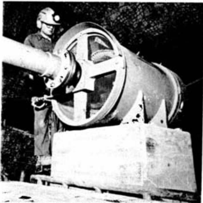
Karl Neuman, Creighton Mine ventilation assistant, records the motor nameplate data for future reference. This 450 h.p. motor turns the shaft at some 880 rpm.
